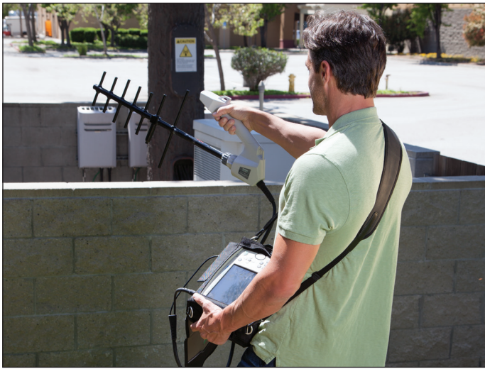
BTS Master MT8220T utilizing Handheld InterferenceHunter™ MA2700A
